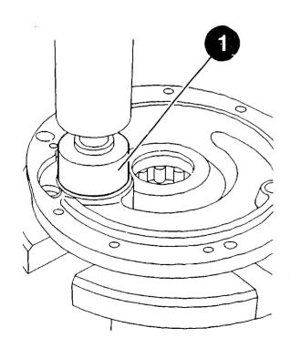
CHECKING/REPAIRING COMMUTATOR END SHIELD
